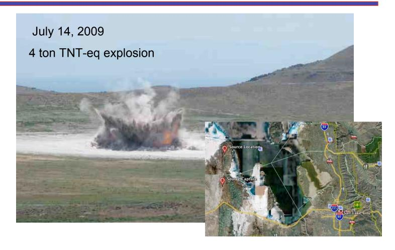
4, 20 and 80 tons-TNT equivalent explosions at the Utah Testing and Training Range (UTTR), as part of the Trident missile disposal program.
