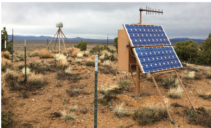
FIGURE 2. GPS Station P073 in TwinSpring, Nevada. The GPS antenna on the left is anchored to the ground. Communication equipment, solar panels, and equipment enclosure with GPS receiver and batteries are on the right. Source: EarthScope Consortium
