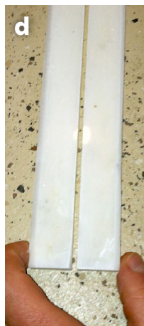
FIGURE 5. (a) Marble tongs and (b) rubber band and mini compression spring. (c) Stress is applied to the cut end of the marble tong, deforming the marble when closing the tongs. (d) When stress is removed, the marble springs back as the stored energy is released.
