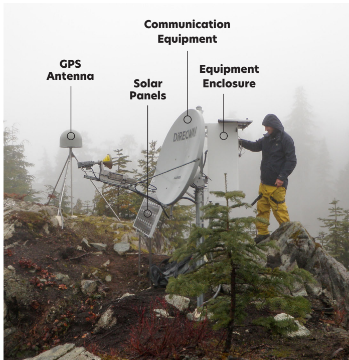
FIGURE 2. GPS Station P443 in Marblemount, Washington. The GPS antenna on the left is anchored to the ground. Communication equipment, solar panels, and equipment enclosure with GPS receiver and batteries are on the right. Source: EarthScope Consortium
