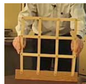
Left: Basic 4-cell model. Right: Expanded 9-cell model demonstrated in this video: Build a Better Wall: How can we make a building more earthquake proof?
