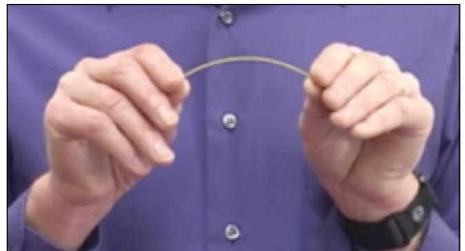
Figure 4: Spaghetti demonstration of elastic strain.
