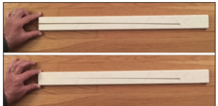
Figure 5: Rock demonstration of elastic strain. Here we used a piece of marble threshold slit with a rock saw.
