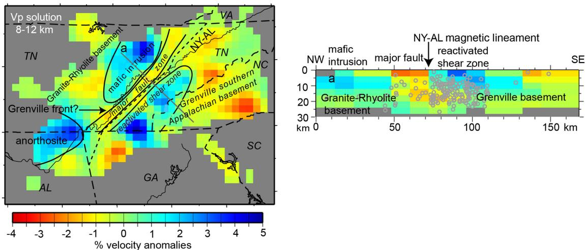
ETSZ seismotectonic model. Earthquakes occur in the “reactivated shear zone” bounded to the NW by the New York-Alabama magnetic lineament. The major basement fault extends to at least 24 km depth and is interpreted as a preserved portion of a transform fault accommodating along-strike migration of the Amazon craton relative to Laurentia during the Grenville orogeny.
