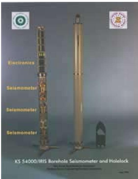
**Figure 5:** Photograph of a modern three-component borehole seismometer. Three seismometers are stacked inside a tube with electronic circuitry. The instrument is encased in a vertical drill hole. The seismometers detect the motion and send a signal to the seismograph to be amplified and recorded
