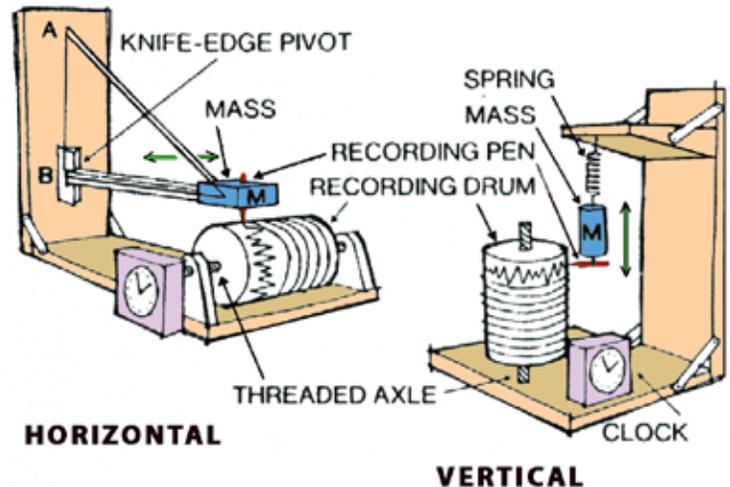
**Figure 2**—The horizontal seismograph (above left moves only in the horizontal plane. Vertical seismographs ((Figure 1 and above right) use a "soft" link between the earth-anchored instrument and the suspended mass. In this design, the mass hangs from a spring, which absorbs some of the motion and causes the mass to lag behind actual motion. (From USGS.gov.)
