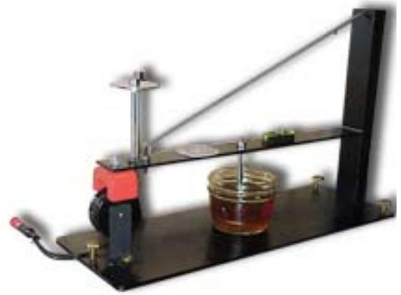
**Figure 6:** Photograph of a simple AS-1 vertical seismometer used in IRIS' *Seismographs in Schools* program <http://www.iris.edu/hq/sis>
