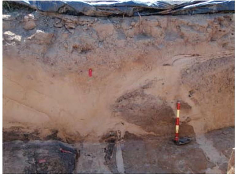
Large liquefaction features resulting from strong earthquake-shaking in the New Madrid seismic zone. Exposed through trenching, the wall and floor of the excavation reveal a portion of a sand blow and related sand dikes. The degree of soil development above and within the sand blow suggest that the earthquake that formed this feature occurred prior to the 1811-1812 New Madrid earthquakes. Photo by Martitia Tuttle.
