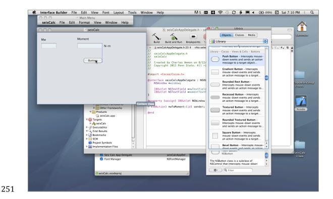
That's our simple user interface – we have all the objects in position. Three labels and three control objects (two text fields and one push button). All that remains is to connect this interface to the object references in our source code. We are going to connect the text fields to our two IBOutlets and set the push button so that is executes our IBAction function to compute the moment from the Mw.
