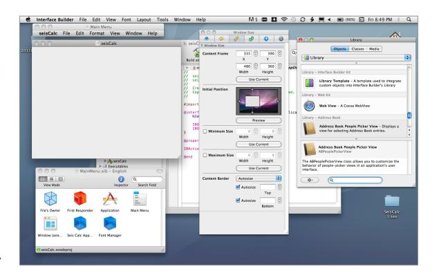
The window on the lower left shows the objects that are contained in the MainMenu.xib file. The window in the middle is the Inspector, which allows you to customize objects that you add to our interface. The Inspector shows information about our application window because I clicked on the seisCalc window.
