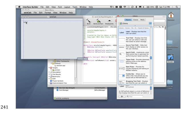
Now drag a Text Field item from the library to the seisCalc window and align it below our label. This text field is where the user will enter the value of moment magnitude (Mw) that we will use to compute the seismic moment.
