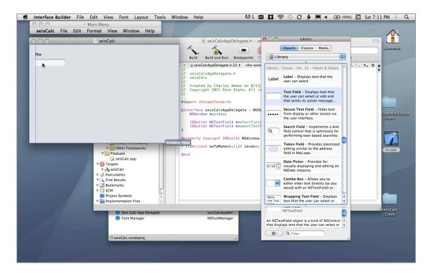
Repeat the process to create a Label and Text Field for the seismic moment Add a third Label to provide the units for the seismic moment value. Now change the text in the search field of the Library window to "button" (without quotes). Then drag a Push Button object from the Library palette to the application window. Double click the button to rename it "Calculate".
