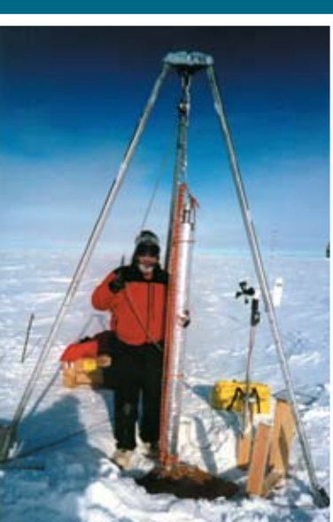
Kent Anderson (ASU) preparing to test a KSS4000 for deployment in the ice at the South Pole.
