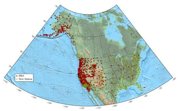
Distribution of PBO station (red) and extra stations to be added to PBO processing (yellow). The new stations NGS CORS, SCIGN, SOPAC, and local networks, will expand geodetic coverage across North America.
