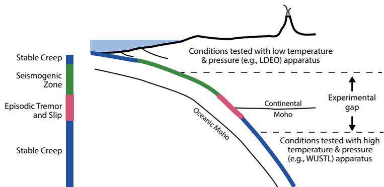
The distribution of fault slip behavior in a subduction zone and the conditions that are achievable in an experimental apparatus. There is a gap in experimental capabilities between the downdip transition from seismic slip to stable creep. *Modified after Scholz (1998)*
