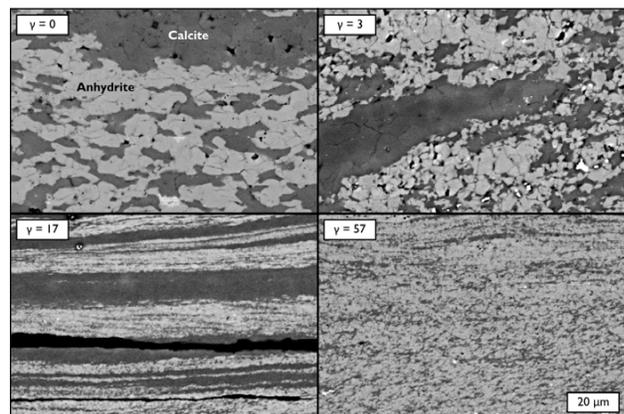
Rock deformation experiments are used to study connections between microstructural evolution and strength over a wide range of deformation conditions, including variations in stresses, strain rates, temperatures, pressures, and fluids. The photos show a sequence of deforming calcite-anhydrite mixtures from low to high strain. *From Cross and Skemer (2017)*
