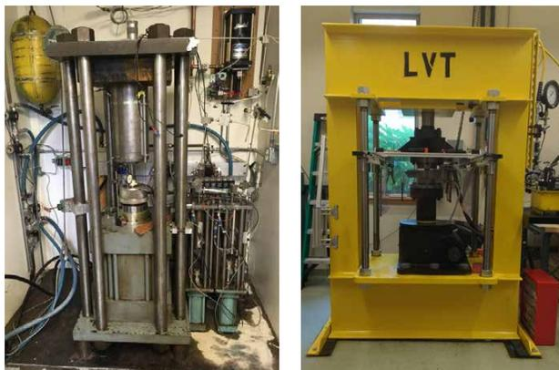
(left) The triaxial apparatus at Lamont-Doherty Earth Observatory is used to study rheology at low pressure and temperature. (right) The large volume torsion apparatus at Washington University in St. Louis is optimized for mantle conditions. *Photo credits: (left) Philip Skemer and (right) Heather Savage*
