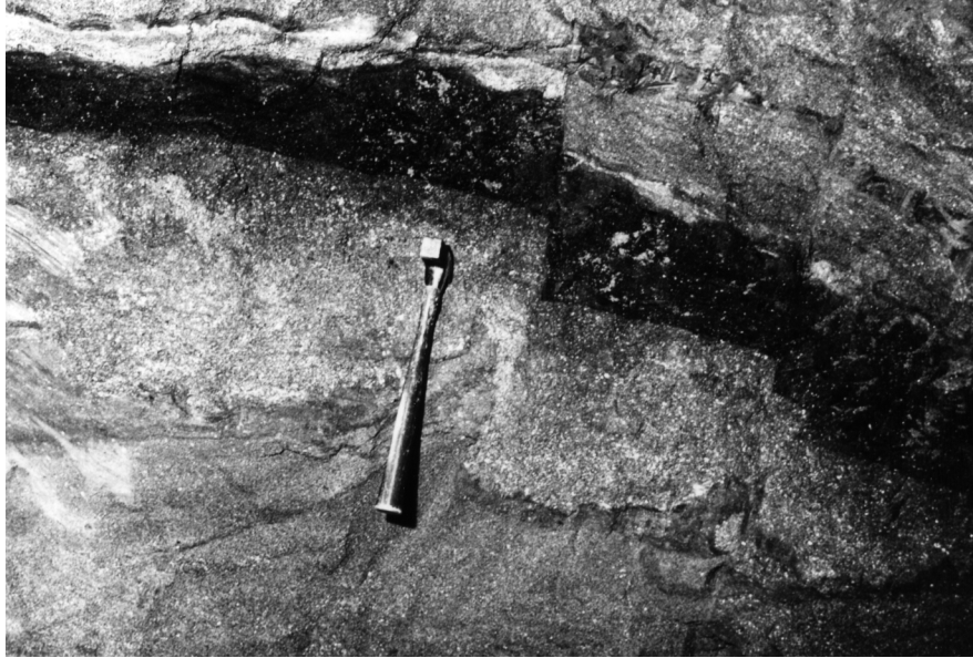
Figure 3. Shaft fault as seen in vertical section during excavation of reactor shaft at Bodega Head site. In Quaternary beds, the maximum observed vertical separation on the fault was 0.36 m; a strike-slip component was recognizable but was of unknown amount. In the granitic bedrock the observed strike-slip component was 7.3 m and the fault was 0.6 to 3.0 m wide. Photograph by Julius Schlocker, U.S. Geological Survey, 1963.
