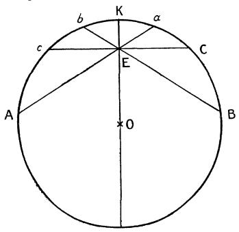
we shall assume that cC is an arc of  $17^{\circ}\cdot 1$  so that a P wave starting from a deep-seated focus E along EC will be reflected at C so as to strike the surface again at  $C_1$   $C_2$   $C_3$  . . . where  $CC_1 = C_1C_2 = C_2C_3$  . . . =  $17^{\circ}\cdot 1$ ; and after five such reflections will reach a distance  $\Delta$  from K (the epicentre) equal to  $5\cdot 5\times 17^{\circ}\cdot 1=94^{\circ}$ . The whole time required would be, with adopted tables,
