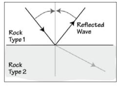
When a wave encounters a change in material properties (seismic velocities and or density) its energy is split into reflected and refracted waves.
