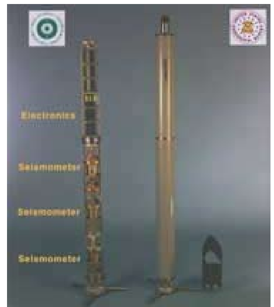
Figure 5 : Photograph of a modern three-component borehole seismometer. Three seismometers are stacked inside a tube to measure movement in 3 axes: x, y, and z. The instrument is encased in a vertical drill hole. The seismometers detect the motion and send a signal to the seismograph to be amplified and recorded by computers.
