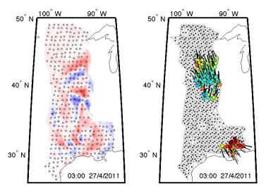
Caption: (left) Pressure data, recorded on LDM channels and bandpassed from 2-4 hours, are interpolated across the TA.
