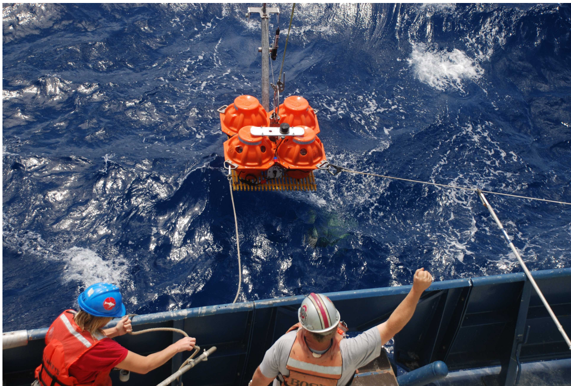
Figure 2. Bosun Wayne Bailey directs the retrieval of a OBSIP broadband OBS while SSSG tech Allison Heater attaches a tag line.
