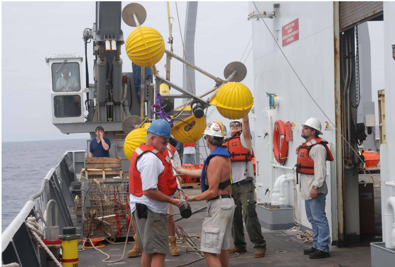
Figure 7. Geodesy Tripod C2 is recovered by Rob Handy and the Thompson's crew after it failed to establish communications with other instruments at its first deployment location.
