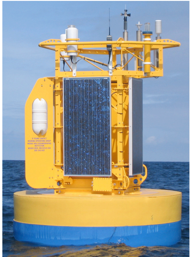
Fig. 3. Buoy with solar panels, meteorological sensors and antennas.
