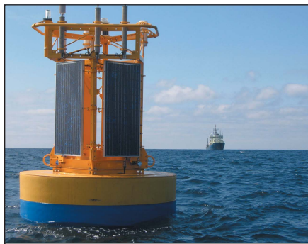
Fig. 2. A 2.7-meter-diameter surface buoy deployed at the Nootka observatory with solar panels, meteorological sensors, and antennas mounted on an aluminum frame atop the float. A universal joint between the buoy and the mooring provides for up to 60° of motion in two planes, protecting the conductors from bending strain produced by the motion of the buoy in severe sea states.
