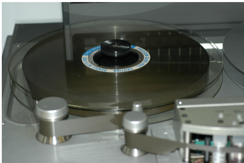
A view of the operating area (above) Use of precision glass reels (and some tape damage, below).
