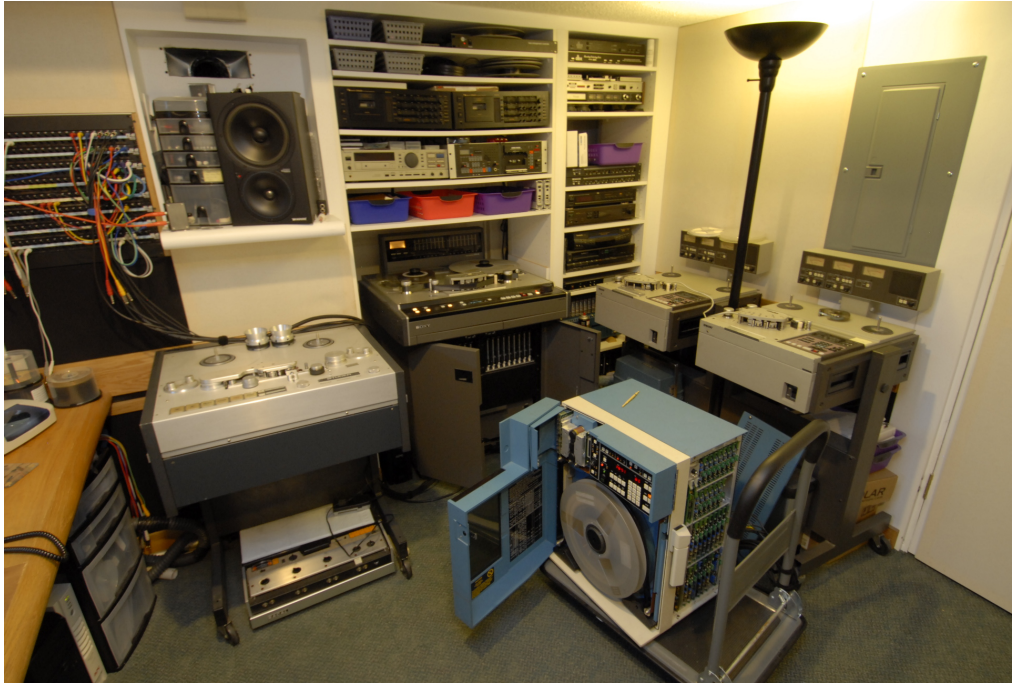
Equipment layout-blue machine is Honeywell 101, machine to its left and rear with doors open is the Sony APR-16 which was used for winding the tapes. Below is a view of the custom demodulator “black box” (lower right) connected into the studio patchfield.
