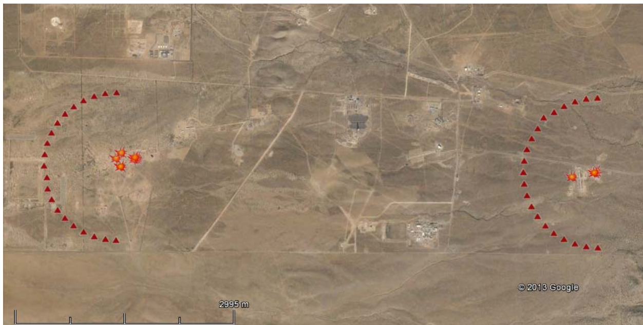
Figure 1. Map of Array 1 seismic stations (triangles) and shot locations (orange flames) on KAFB. (Google Earth Background).
