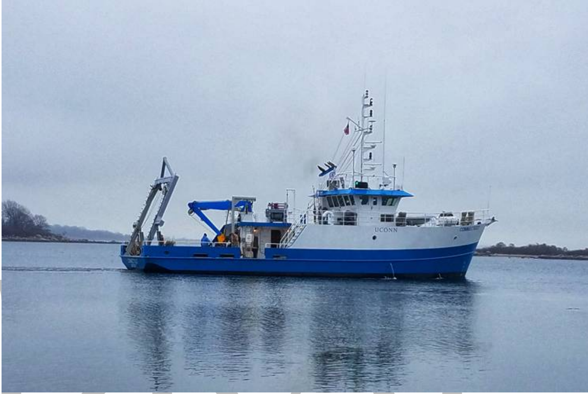
Figure 3. R/V Connecticut after recent lengthening to 27 m (90 ft). Image from https://www.marinetechnews.com/news/lengthened-research-vessel-556363 .
