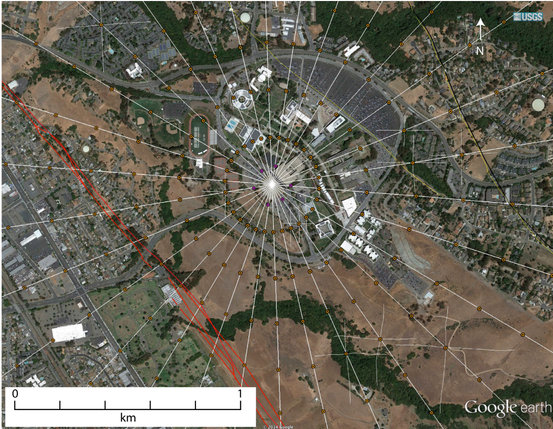
Figure 3b. Location of the radial/circular (gold), near-source (magenta), and fault zone (cyan) Arrays of the EBSE. The red lines show the active traces of the Hayward Fault. Other Holocene or Quaternary faults are shown by the yellow lines.
