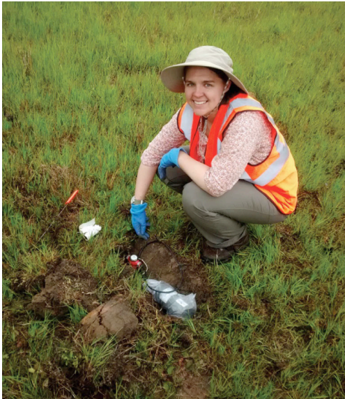
Fig. 8: ( top left ) Chastity Aikens (Ga. Tech) plants a Texan and levels the geophone.
