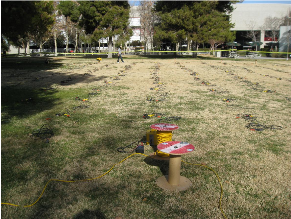
Figure 2. Layout of cable and geophones for Surfbar-2 test on 15 Jan (View to the north).
