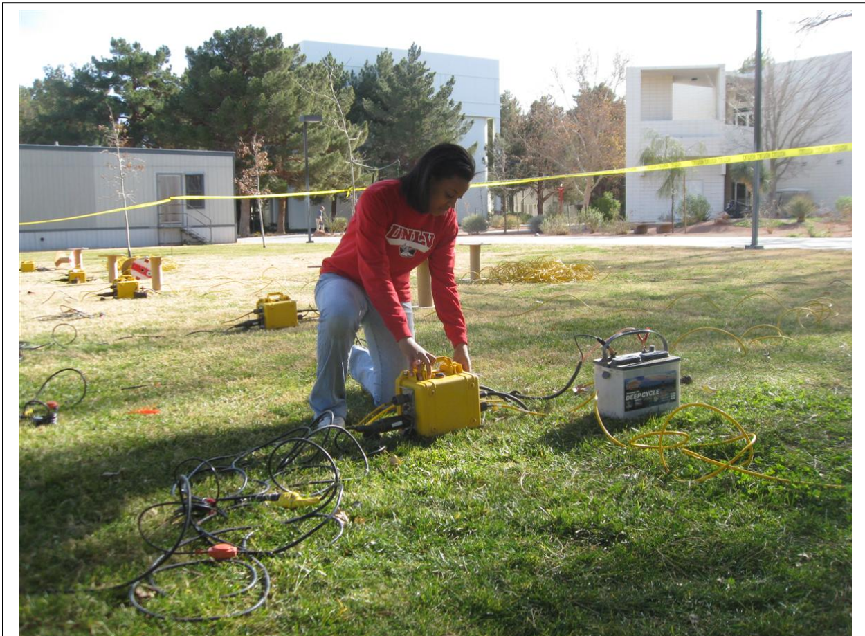
Figure 3. Geodes connecting geophones
