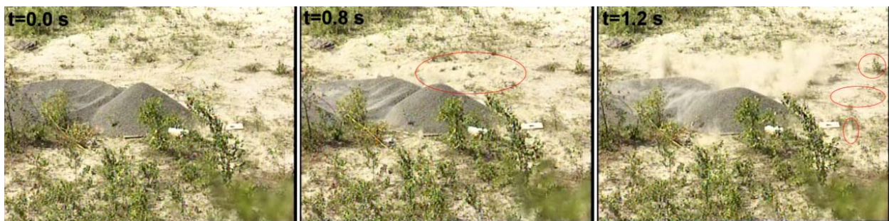
Figure 23. Digitized still images of the Shot 1 detonation. Note the two fractures developing after 0.8 s and the further fractures after 1.2 s in the red ellipses.
