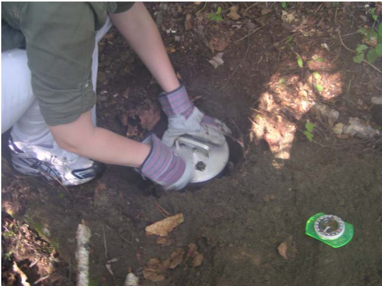
Figure 12. Example of orienting to true north and leveling an L4-3D sensor on the NE line.
