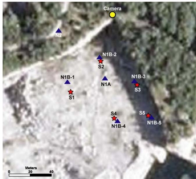
Figure 6. Test site station N1 (blue triangles) and shots (red stars). N1 consisted of two Endeveco accelerometers. N1A remained stationary for all 5 shots, while N1B moved to be less than 5 m from each shot. Station N2 and the camera are also shown on a hill overlooking the test site. (Google Earth Background)
