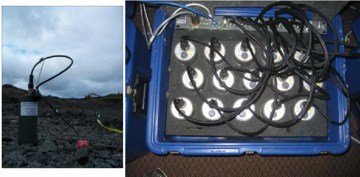
Figure 13. (Left) RT-125 “Texan” seismic recorder and attached 4.5 Hz vertical spike geophone (orange). For the experiment, the recorder was placed in a plastic bag, laid on its side in a trench, and everything was buried. (Right) Texans in their carrying crates being programmed prior to deployment.
