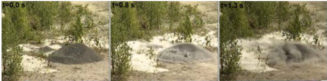
Figure 27. Digitized still images of the Shot 4 detonation. This shot produced significantly more dust than Shots 1-3. There may be small amounts of gas release in the gravel pile after 0.8 s, but there were no large fractures observable on the video like for Shots 1 and 2.
