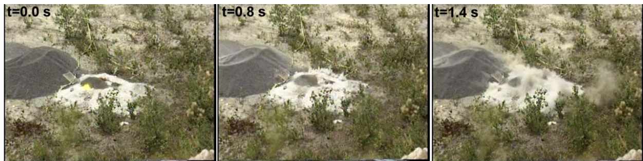
Figure 25. Digitized still images of the Shot 2 detonation. Three fractures develop in the white granite floor at 0.8 s and a larger opening releases a plume of gases to the right of the floor at 1.4 s.
