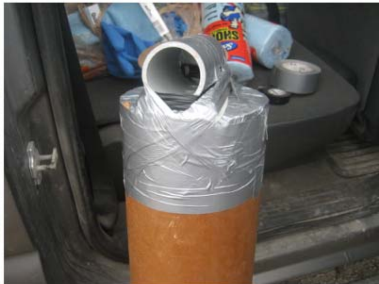
Figure 16. COMP B charge and the tube taped on to hold the detonator.
