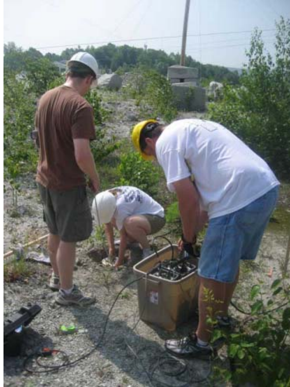
Figure 8. Example of near-source instrument installation. Katherine Murphy levels and orients a TerraTek accelerometer to true north while Sam Huffstetler installs the Reftek 72A-08 digitizer and battery.
