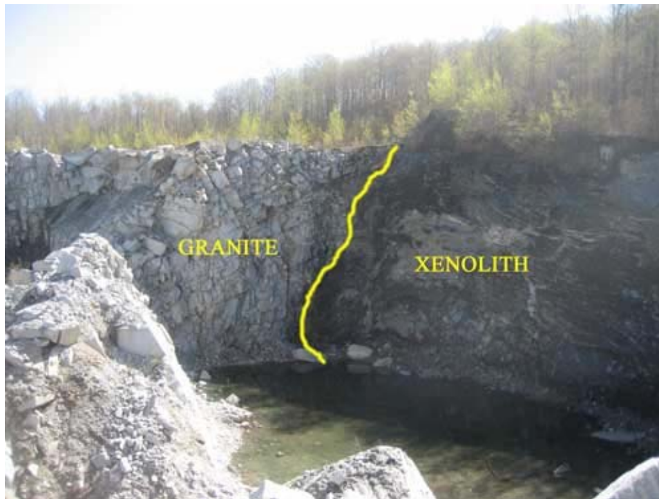
Figure 5. Photo of the highly-fractured nature of the granite at the alternative test site (see Figure 4) and a contact with large xenoliths at the abandoned test site.
