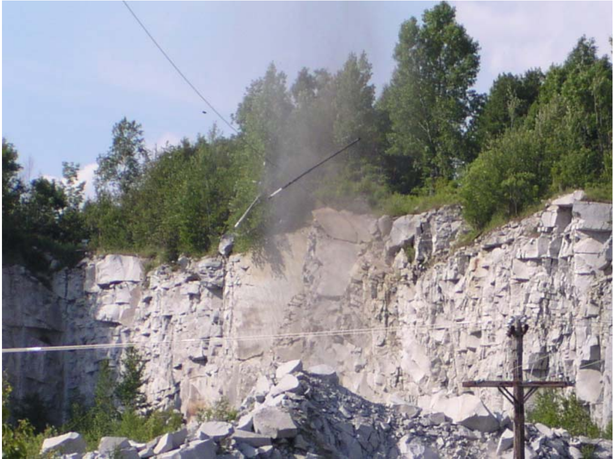
Figure 30. PVC pipe breaking on guy line during free fall after being ejected from a nearby borehole during Shot 5.
