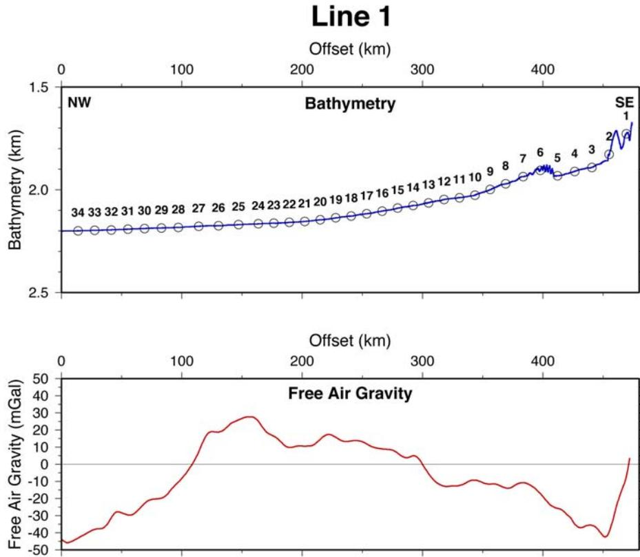
The upper panel shows bathymetry derived from a shipboard echosounder with the locations and position numbers of OBSs. The lower panel shows satellite gravity with free air corrections.
