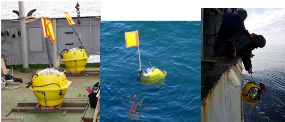
**Figure 4: OBS ready for deployment (left), awaiting recovery (centre) and being hauled aboard (right)**
