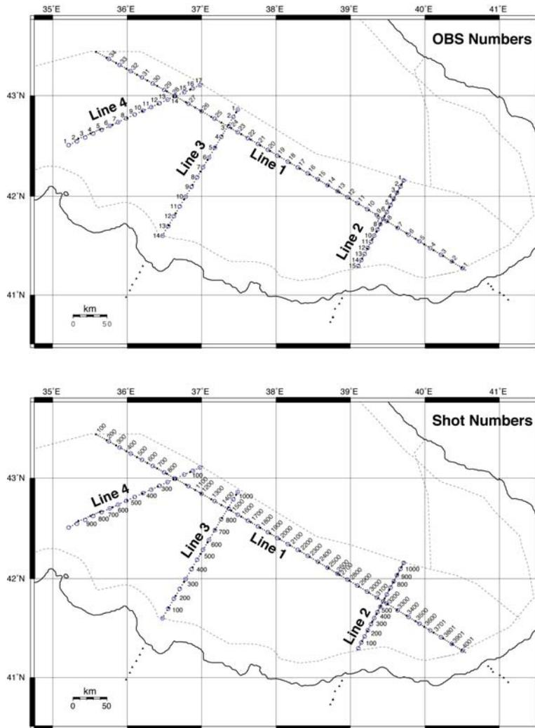
**Figure 6: OBS positions on the wide-angle seismic profiles (above) and shot numbers along the profiles (below)**
