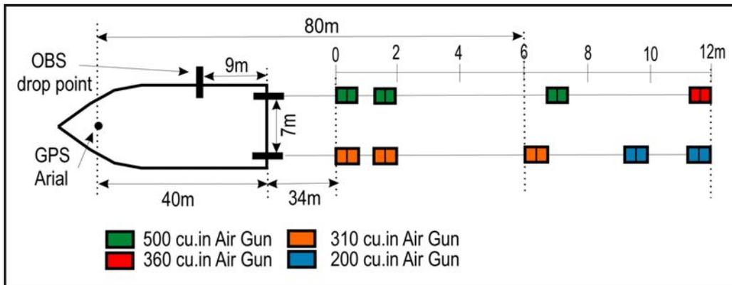
**Figure 3: Geometry of airgun array. Guns were towed at ~9 m depth**
