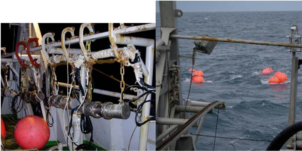
**Figure 2: Port airgun string (left) and deployed airgun source (right)**
