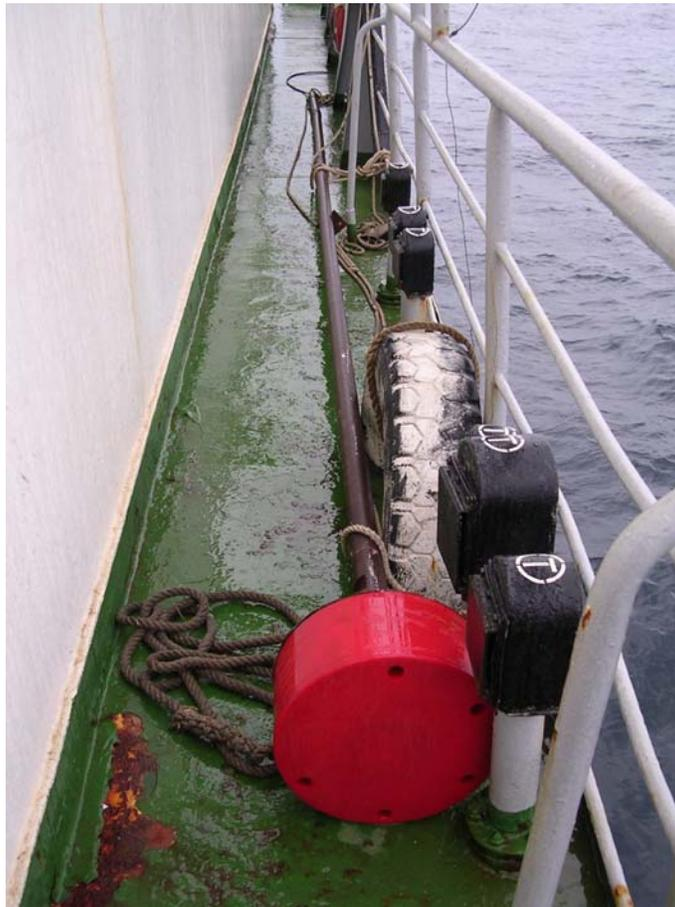
**Figure 1: Echosounder with its pole**
