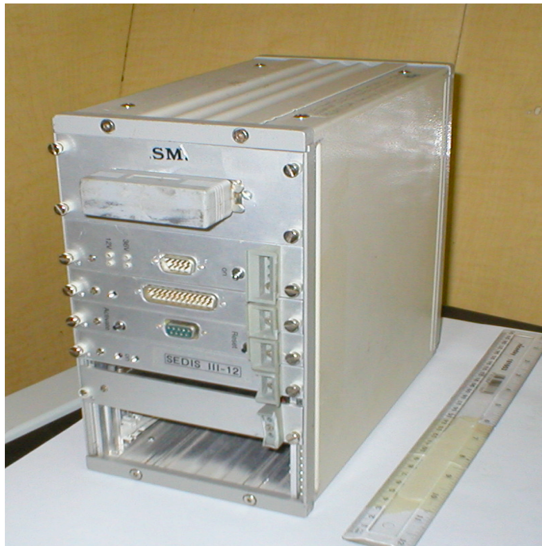
Fig 3. 6 channels portable seismic recording unit – Seids –III is ideal for offshore and on-shore applications
