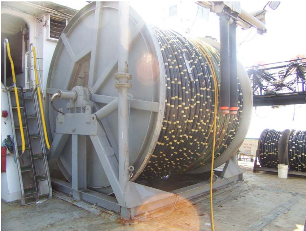
Figure 10. The Ewing 's 480 channel hydrophone streamer on the fantail. Replacement sections can be seen in the background and digitizing cans can be seen spaced along the streamer (these sum the acoustic signals and send them up the streamer to the recording systems on the vessel).
