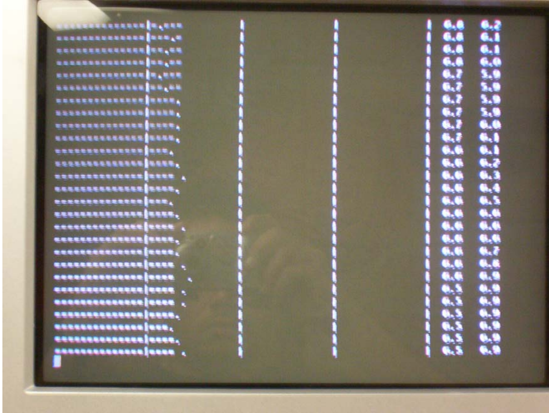
Figure 4. Screen on the Ewing that displays the wind data. The bars along the left show the 90 minute running average of the wind and become bright if the 90 minute average exceeds 17 knots. The numbers on the right are the 15 minute and 90 minute running averages. The vertical dashed lines are at 5 knot intervals.
