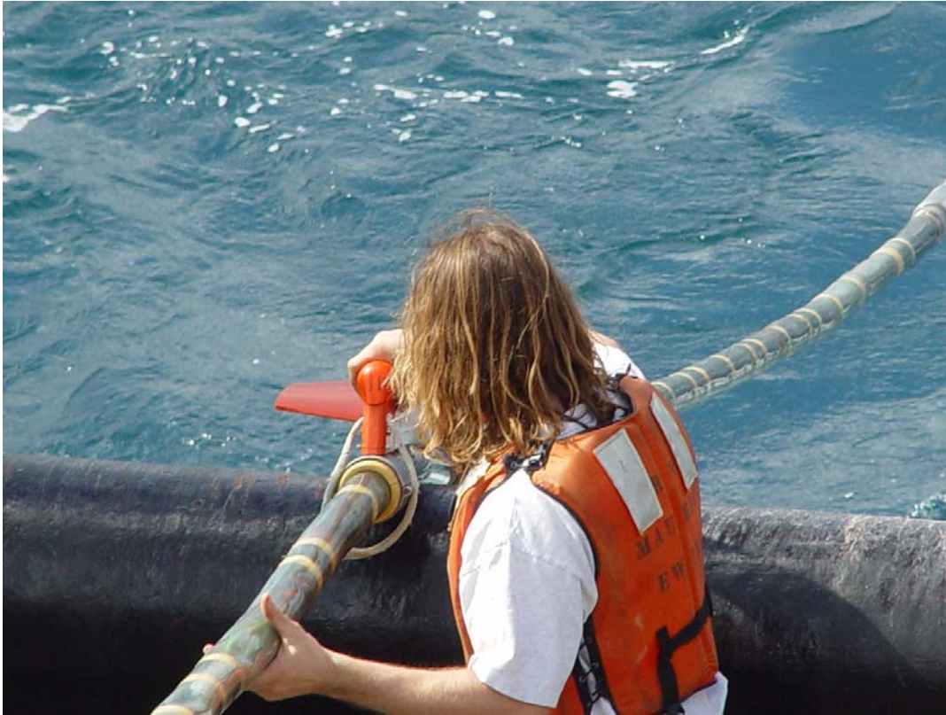
Figure 11. Compass bird being clipped on the streamer during deployment.
