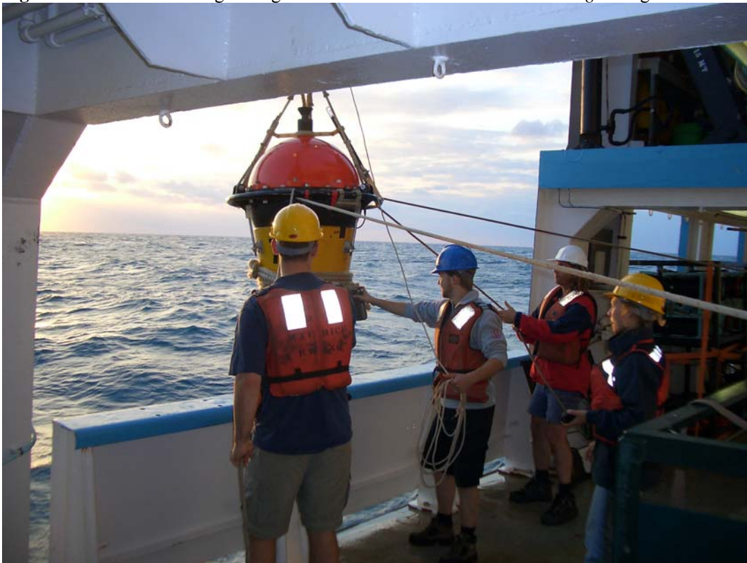
Figure 15: OBS of the DOBS design being launched during cruise EW0501.
