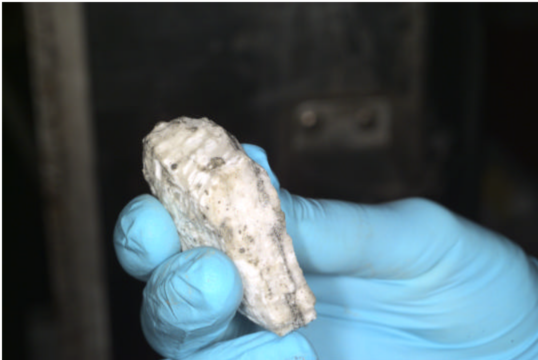
Gas hydrate samples retrieved from cores at Site 1244 during Leg 204. These solid pieces probably formed within veins formed within faults.
