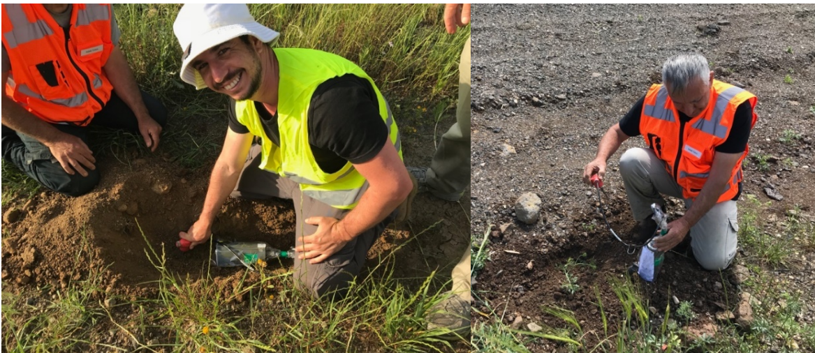
Figure 6 – Deployment (left) and recovery (right) of a Texan receiver unit.
