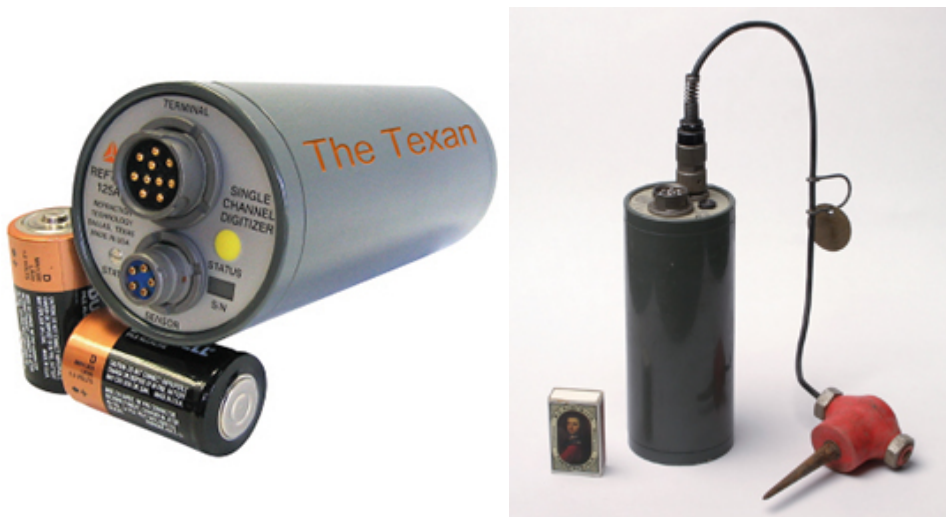
Figure 3- Texan RT125A (left) and Texan connected to Geospace GS-11D 4.5 Hz geophone.
